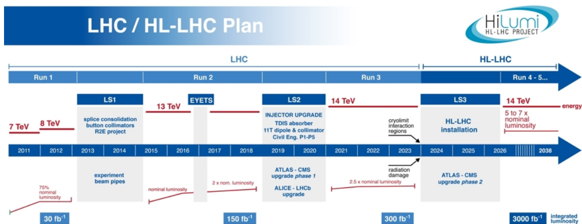
Figure 1: LHC timeline showing the energy of the collisions (red line) and luminosity (green lines).
